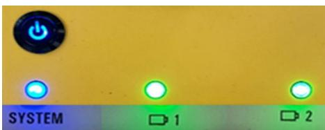
4. Press the O/I button next to the battery compartment to start up the DS4000 antenna.
